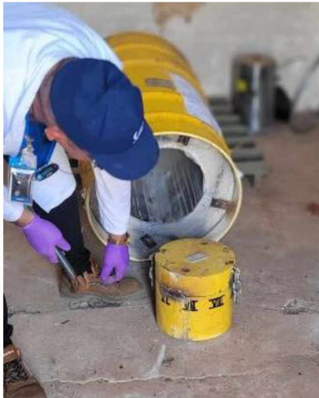
Fig. 1. Tipped over 200-L steel drum with smaller steel cylinder containing the sources removed. Note the hollow concrete cylinder inside the drum.
