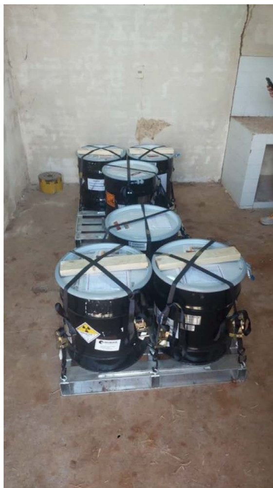
Fig. 4. The six Type A shipping containers, covered, torqued, labeled, strapped, and placed on pallets, ready for transfer to the airport.
