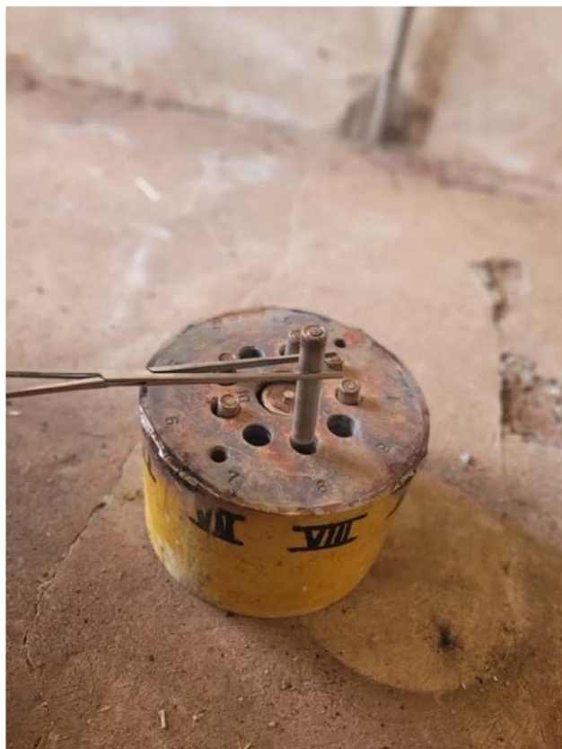
Fig. 2. The six ^{226}\text{Ra} sources (in outer circle) and 116 ^{137}\text{Cs} sources (in center circle) inside the smaller steel cylinder.
