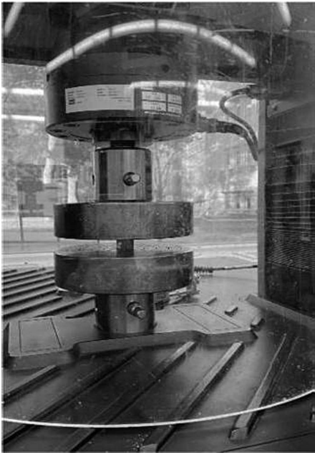
Fig. 2. Bone sample undergoing compressional testing on the UTM. Note the use of acrylic shield to protect personnel from possibility of explosive structural failure of specimen!
